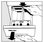
Press down the red release knob and at the same time pull the drawer right out of the machine.
